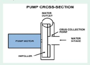
Water is drawn into the pump through a very small gap between the intake pipe and the pump impeller. Even small amounts of debris can plug this gap.
