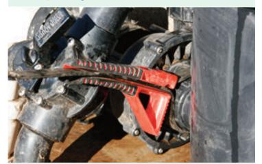
Once the couplings are loosened, the pump is very easy to lift/slide out.
